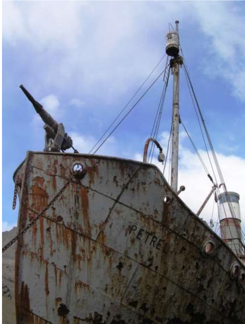
A harpoon launcher rides the bow of the Petrel (photo: Dan Linehan).
